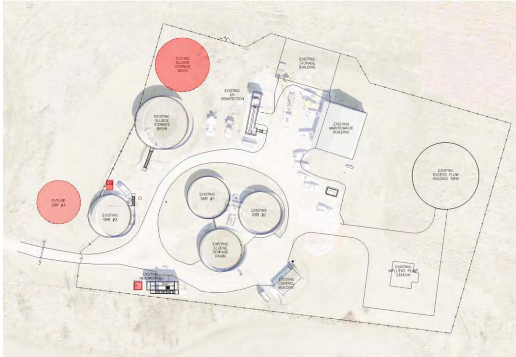
Phase II expansion will require the addition of a fifth and sixth SBR basin. Again, upgrades are required at the influent valve vault and effluent valve vault. Additional bulbs will be added to the UV equipment to increase the design capacity. One more additional sludge storage tank will need to be added to the treatment plant to increase sludge storage capacity.
